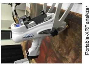
Portable XRF analyzer
